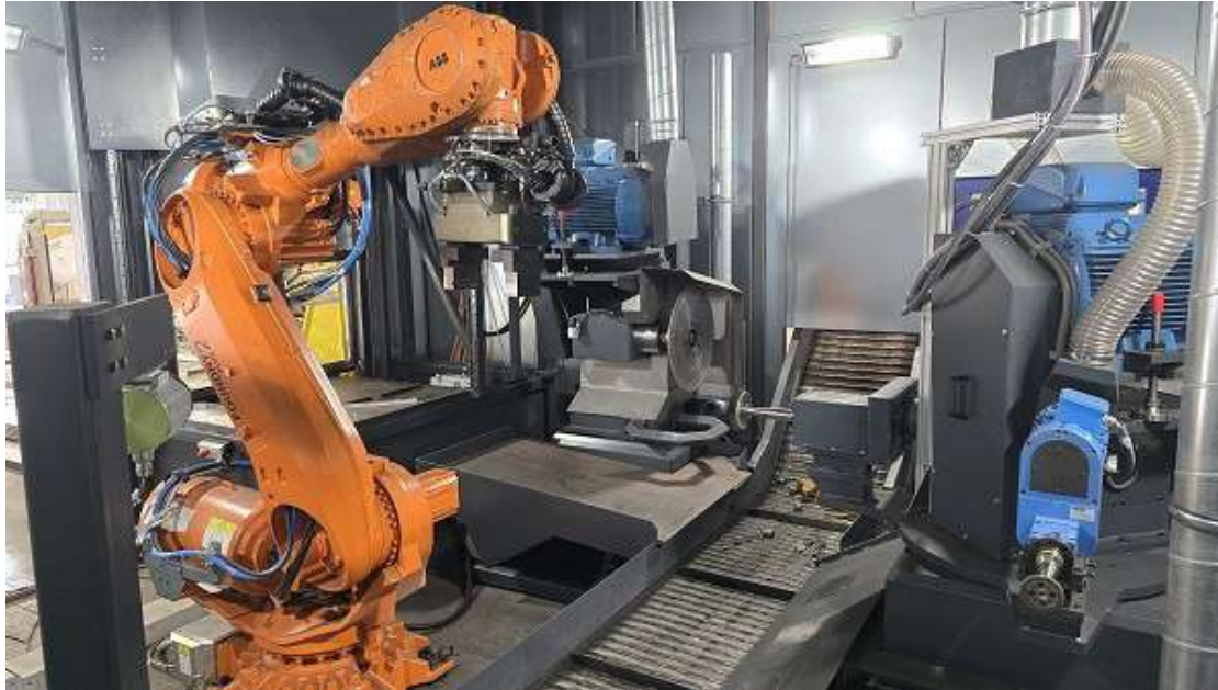
Camera System for 3D-part Recognition and Localization for Picking of unsorted Workpieces for Machine Loading and Automation
